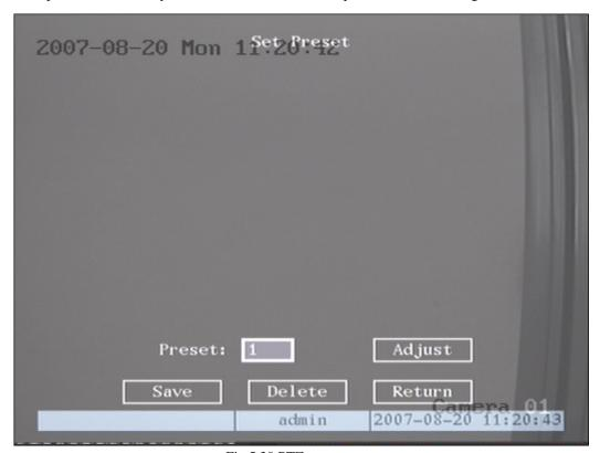
Fig 5.30 PTZ preset setup
